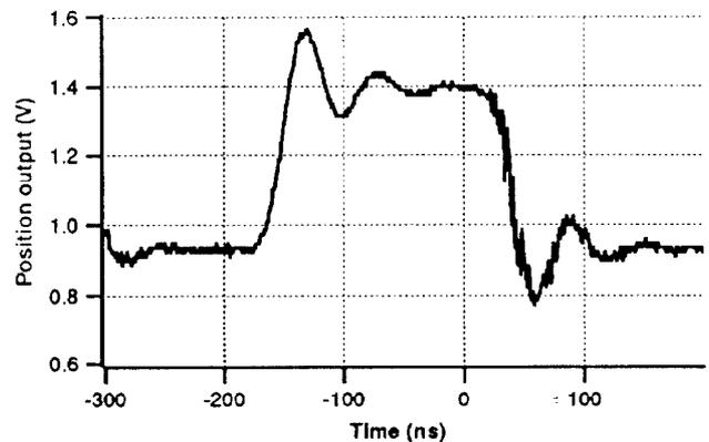
Figure 5. Module's response to simulated beam displacement.
