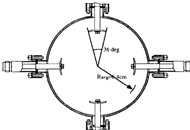
Figure 2. End view of beam position monitor.
