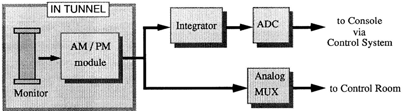
Figure 3. Block diagram of beam position monitoring system.
