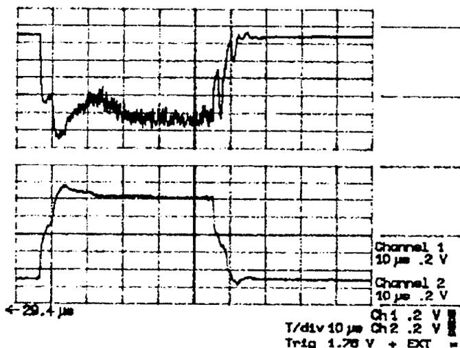
Figure 7. Analog signals: horizontal on top, vertical on bottom. 100mV corresponds to a 1mm displacement.
