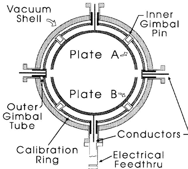
Figure 2. Double-gimbal beam position monitor.
