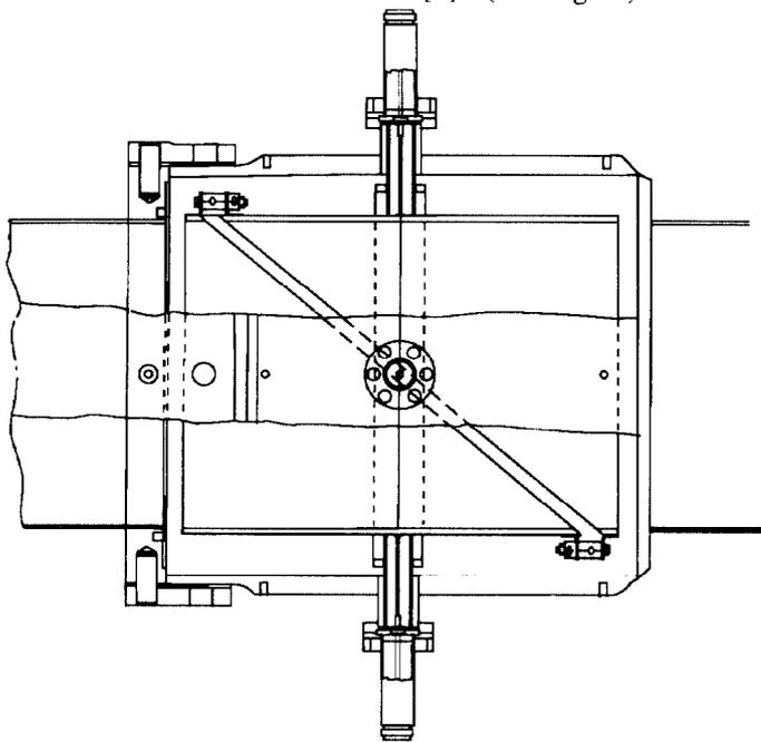
Figure 1. Beam position monitor (longitudinal view).
