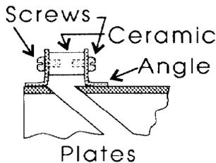
Figure 3. Split-cylinder assembly.
