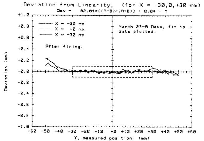
Figure 5. Typical scan wire measurement results.
