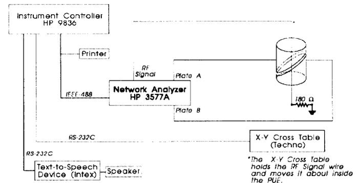
Figure 4. Set-up for the scanned wire measurements.
