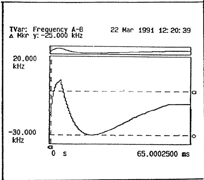
Figure 3. Open Loop Frequency Error
