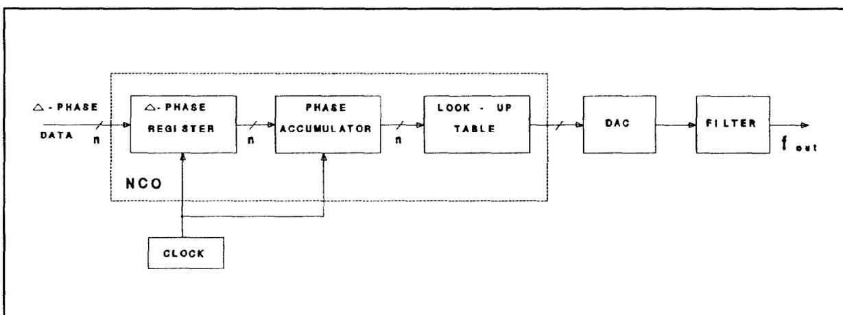
Figure 1. DDS Block Diagram
