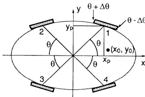
Fig. 1: Geometry of the beam chamber and the pickup electrodes.
