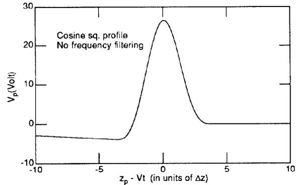
Fig. 2: The electrode signal  $V_p$  as a function of time  $t$  without frequency filtering.  $z_p$  is the electrode center coordinate and  $\Delta z$  is half the longitudinal size.
