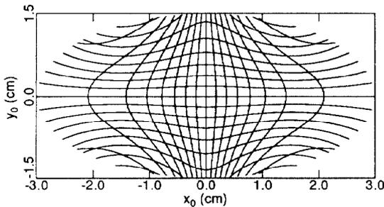
Fig. 4: The contour plotting for  $X_0 = \Delta_x/\Sigma$  and  $Y_0 = \Delta_y/\Sigma$  for the elliptic beam chamber.
