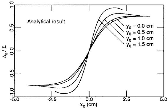
Fig. 3: The ratio  $\Delta_x/\Sigma$  as a function of the beam position  $x_0$  for several cases of  $y_0$ .
