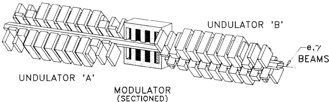
Figure 1: Conceptual illustration of the crossed-undulator source.
