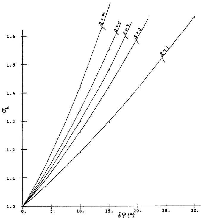
Figure 3. Standing wave ratio at hybrid input plotted against tuning angle difference for various coupling coefficients.
