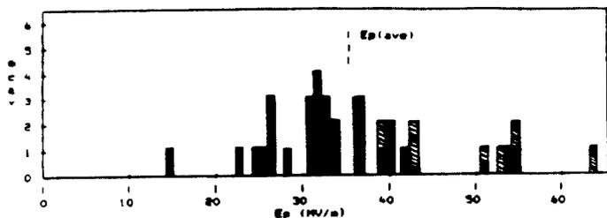
Fig. 1. Distribution of 3 GHz cavity tests related to the maximum peak electric field achieved. ▨ = runs with modified chemistry, ▤ = standard 1,1,1 chemistry. For the cavity geometry,  $E_{peak}/E_{accel} = 3.64$ . Cavity  $Q_0 = 4 \cdot 10^{10}$  at 1.8 K. Total of 36 runs on 9 cavities.
