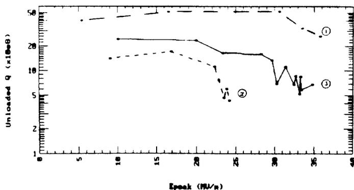
Fig. 3. Comparison of tests after different acid treatments
