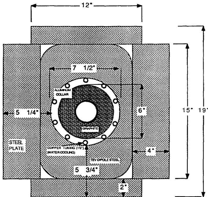
Figure 1. Cross section of the Absorber. From reference[2].
