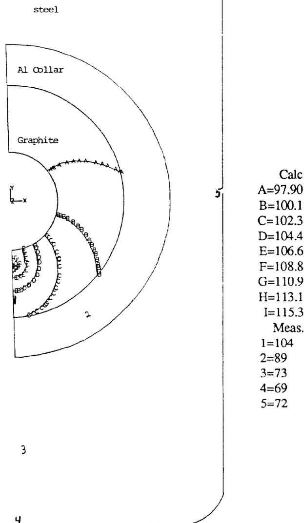
Figure 3. Calculated and measured temperature distribution for the steady state case. All temperatures in degrees C. From Ref[2].
