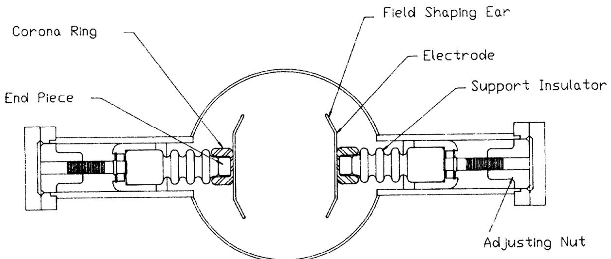
Figure 2: End view of pinger electrode.
