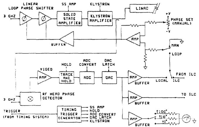
Figure 2. Block Diagram of the Phase Servo Signal Processor
