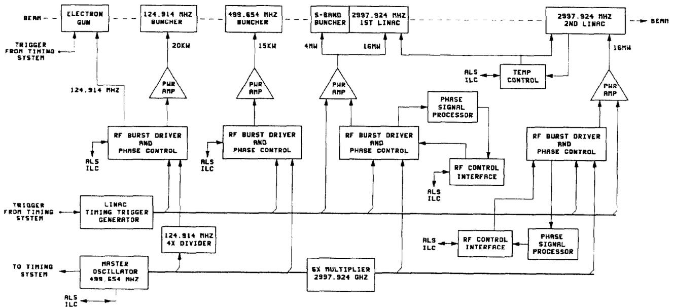
Figure 1. Block Diagram of the ALS Linac RF System
