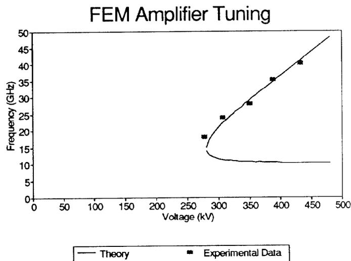
Figure 1: FEM Amplifier Voltage Tuning
