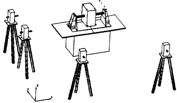
Figure 2: Isometric view of Fiducialization setup for SHR quadrupoles. The survey targets are indicated as dots, the magnet is the rectangular box with the bobbin going through its axis. The four tripods are bolted to the floor.
