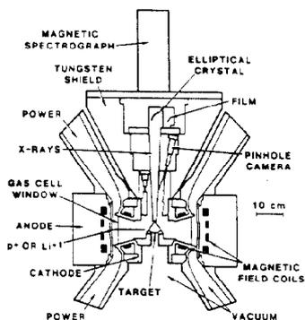
Figure 2. Configuration for target experiments on PBFA II showing upper diagnostics, upper shield, and diode.
