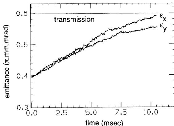
Figure 4: The rms emittance in the LEB as a function of time.
