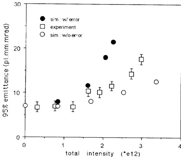
Figure 1: Experimental and simulation results of vertical emittance vs. total intensity in the Fermilab Booster.
