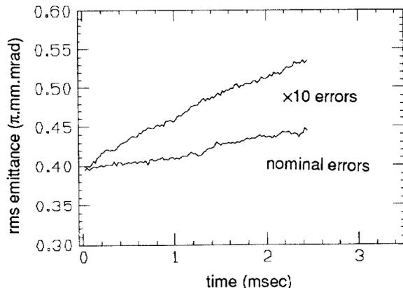
Figure 5: Emittance evolution for different strength of errors.
