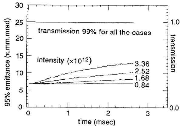
Figure 2: Emittance and transmission as a function of time without errors.
