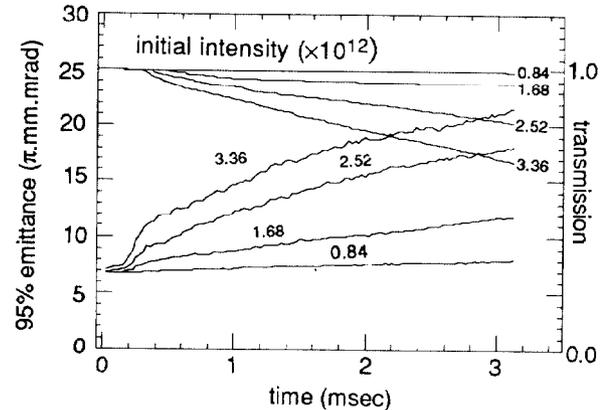
Figure 3: Emittance and transmission as a function of time with errors.
