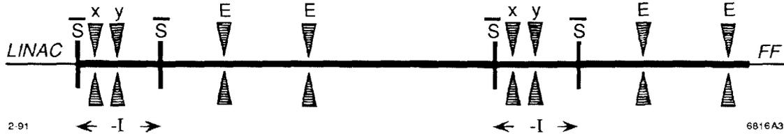
Figure 1. Schematic representation of the collimation systems in the NLC, located between the linac and final focus (FF).  $\bar{S}$  stands for skew sextupole; x,y,E stand for horizontal, vertical and energy scraper respectively.
