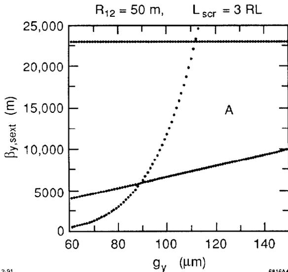
Figure 2. Parameter space for nonlinear collimation with sextupoles.
