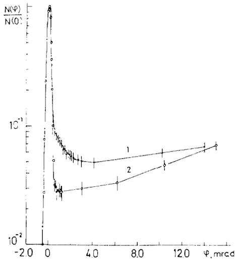
Fig. 2. Plots for the dependence of the number of deflected particles versus the crystal rotation angle w.r.t. the direction of the incident beam.
