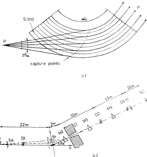
Fig.1a,b. The layout of the experimental equipment. M1-M4 - bending magnets; S1 - a bent single crystal; C1 - steel collimator; D1, D2 and D3 - analog proportional chambers; S1, S2 - scintillation counters (b). Volume capture conditions (a).
