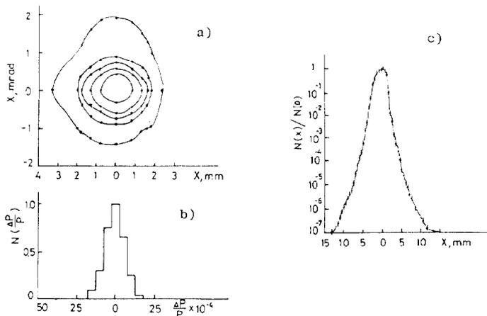
Fig. 6. Measurement results of the incident-on-the-crystal proton beam: emittance. Five closed equipotential lines, starting from the centre, the phase space of the beam at the level 0.75, 0.5, 0.25, 0.1, 0.01 of the maximum density. The following values for the emittance correspond to these figures: (0.26, 0.68, 1.2, 1.6, 4.2)  $\times$   $\text{mm} \times \text{mrad}$ . b) particle spread over momenta; c) beam profile.
