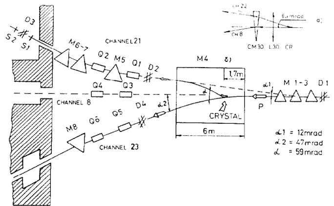
Fig. 4. Location of bent crystals in the proton beam extraction line(a) and in beam line N8 (b) to provide simultaneous operation of beam lines N21, N22, N23.
