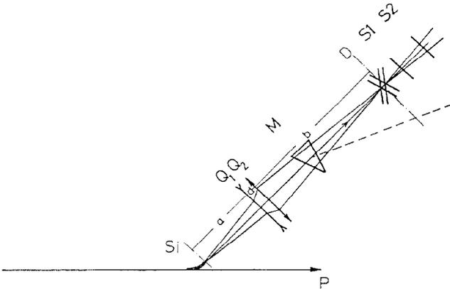
Fig. 5. Beam characteristics measurement scheme Si-bent crystal, D - analog ionization chamber, S1, S2 - scintillation counters, Q1, Q2 - quadrupole lens doublet, M - deflecting magnet (solid lines - the rays - in the horizontal plane, broken line - dispersion).
