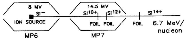
Figure 1. Tandem operating modes during heavy ion operation.
