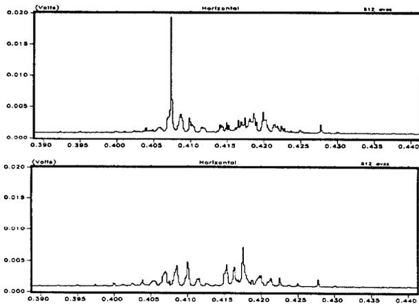
Figure 3: Signals on Schottky detectors with the CDF Toroid on (upper) and off (lower).
