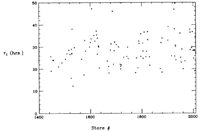
Figure 1: Luminosity lifetimes for Tevatron  $p\bar{p}$  stores from Aug., 1988 to Mar. 1989.
