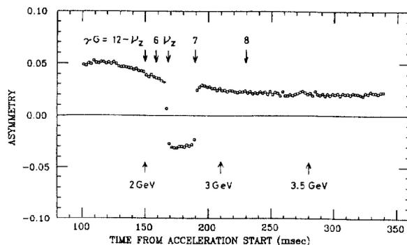
Fig. 2. The asymmetry continuously measured during acceleration.
