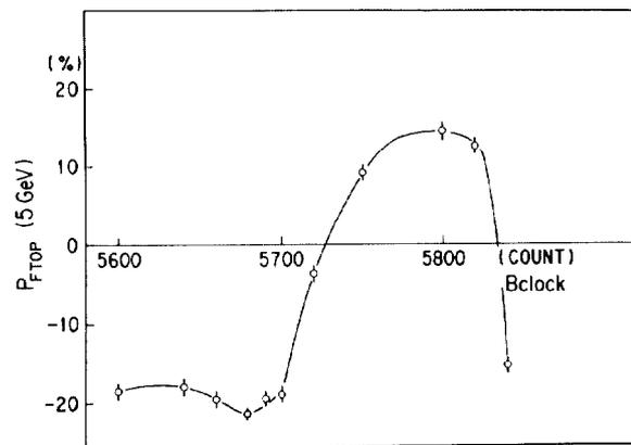
Fig. 5. Correction curve for the  $\Upsilon G = 4+\nu_z$  resonance by the slow passage method.
