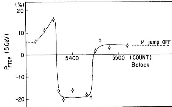
Fig. 4. Correction curve for the  $\Upsilon G = 16-\nu_z$  resonance by the fast passage method.
