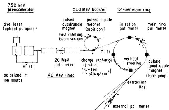
Fig. 1. Equipment designed for the polarized beam acceleration.
