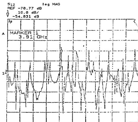
Fig. 10. Value of transmission matrix element between a beam chamber probe and slot probe over the frequency range of 3.5 to 4.5 GHz.
