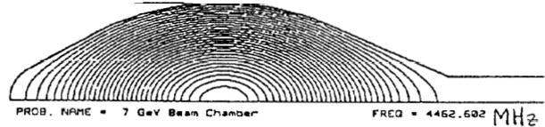
Fig. 2. H-field plot of the dominant  $TM_z$  mode in the beam chamber with longitudinal slot.
