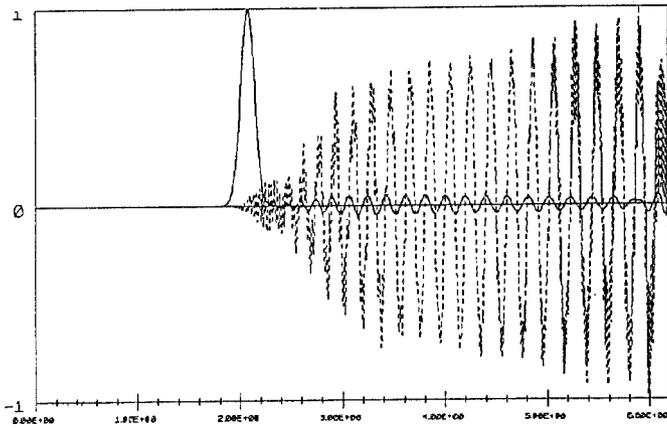
Fig. 4. E-field at the top of slot. The relative amplitude is  $10^7$  V/m.
