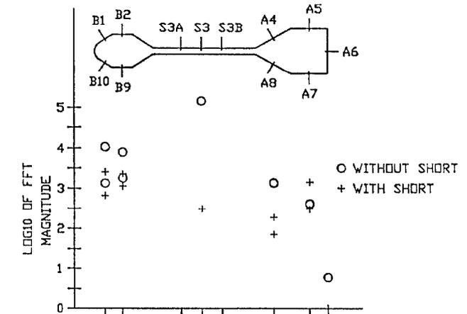
Fig. 8. E-field measurements at 4 GHz with and without slot shorted.
