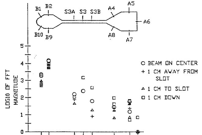
Fig. 7. E-field measurement at 6.5 GHz with beam on chamber centerline,  $\pm 1$  cm horiz. displacement, and 1-cm vertical displacement.
