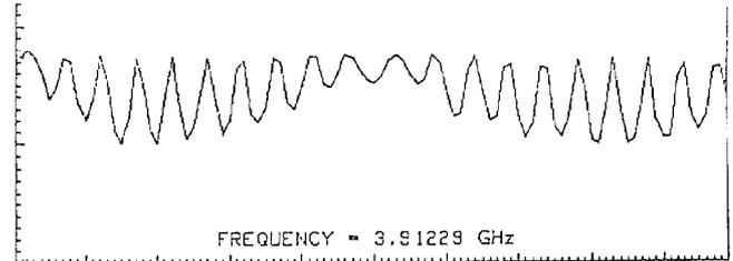
Fig. 11. Value of transmission matrix element between a beam chamber probe and slot probe as a conducting bead is pulled along the z-axis (10 cm per major division).
