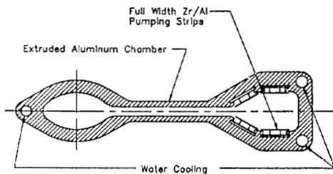
Fig. 1. Cross section of APS vacuum chamber showing beam chamber, pumping slot, and antechamber.
