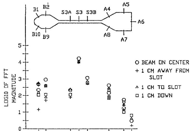
Fig. 9. E-field measurement at 4 GHz with beam on chamber centerline  $\pm$  1-cm horizontal displacement, and 1-cm vertical displacement.
