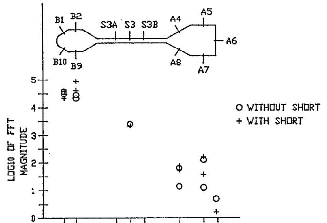
Fig. 6. E-field measurements at 5.5 GHz with and without slot shorted.
