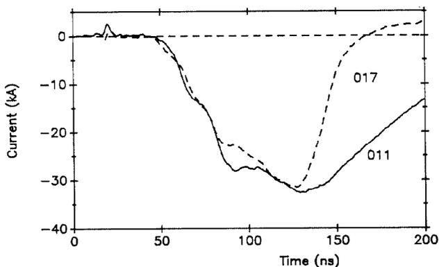
Fig. 2. Entrance (017) and exit (011) current, six cells, 4 cm length.
