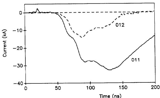
Fig. 3. Net current at end of transport system. a) Shot 011, 6 cells, 4 cm length. b) Shot 012, 1 cell, 24 cm length.
