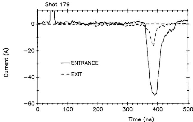
Fig. 5. Net beam current at entrance to and exit from transport system. 1 cell, 48 cm length. 13  $\mu\text{m}$  Ti anode foil.
