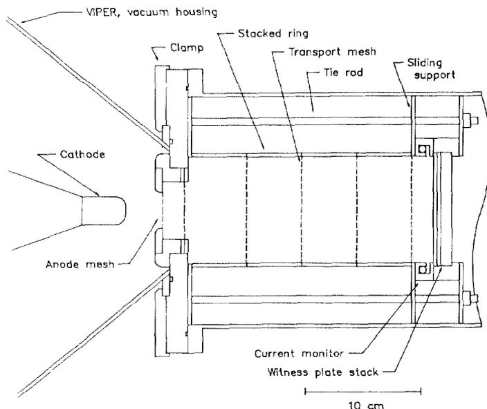
Fig. 1. Scale drawing of the transport hardware on the VIPER generator.
