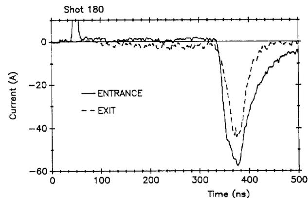
Fig. 4. Net beam current at entrance to and exit from transport system. 16 cells, 3 cm length. 13  $\mu\text{m}$  Ti anode foil.
