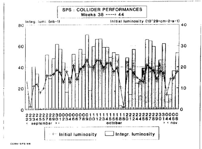
Figure 2: Collider performance 22 Sept-10 Nov 1988 Initial and Integrated Luminosity per store
