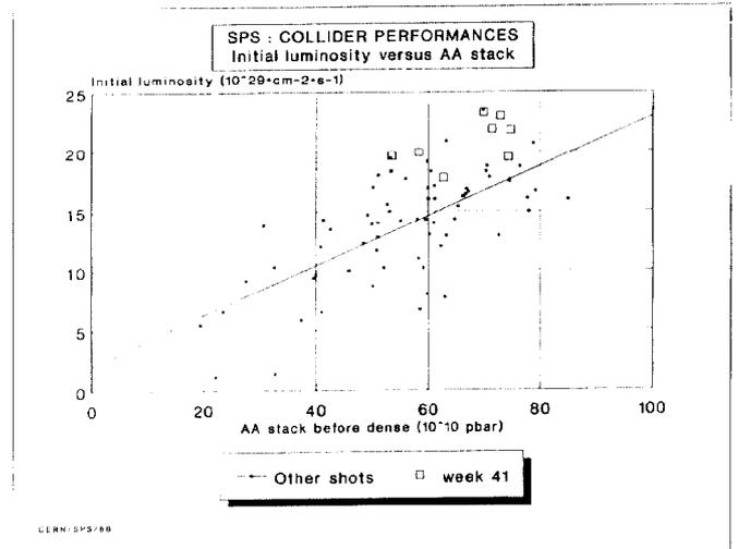
Figure 3: Initial Luminosity, and Transmission as a function of the accumulator intensity
