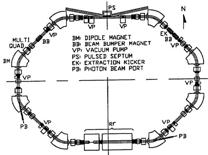
Fig. 2. Layout and Components of the Positron Accumulator Ring.
