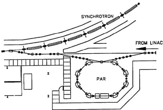
Fig. 1. Location of the Positron Accumulator Relative to the Injector Synchrotron.
