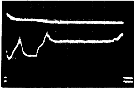
Fig. 7: Beam current (top) and peak-detected wide-band PU for the entire acceleration cycle (100 ms/div.). First loss during and after merging, a few % loss at transition (second peak in bottom trace).
