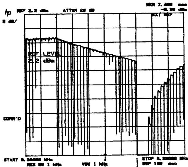
Figure 4. Accumulation of beam at 0.5 Hz using electron cooling. (10 s/div; 5 dB/div). One observes a 20 dB (factor of ten) increase in stored beam after ten injection cycles (last two divisions of the display).
