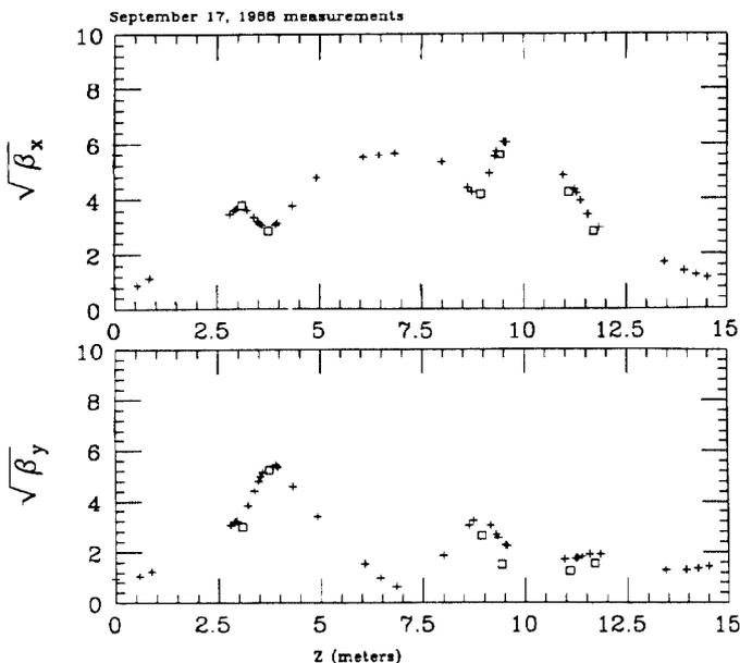
Figure 3. Comparison between measured beta functions (open squares) and calculated values (+ signs) for one sixth of the ring.
