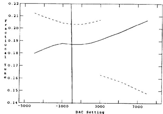
Figure 1. Measured fractional tune vs. quadrupole strength (arbitrary units). The solid line is the "horizontal" and the dash-dot line the "vertical" fractional tune.
