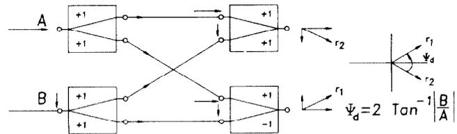
Fig. 2. Operation of the AM/PM converter.
