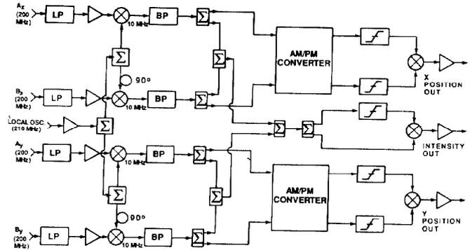
Fig. 1. Block diagram of the beam position-detection equipment.
