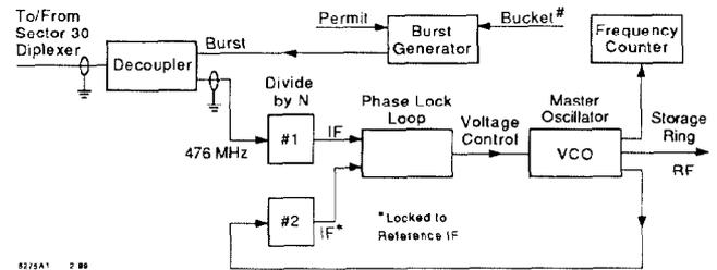
Fig. 2. PEP/SPEAR Phase Lock electronics block diagram.
