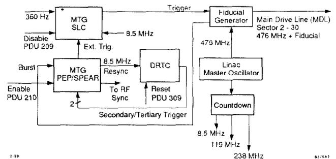
Fig. 3. Linac Fiducial Generation System block diagram.
