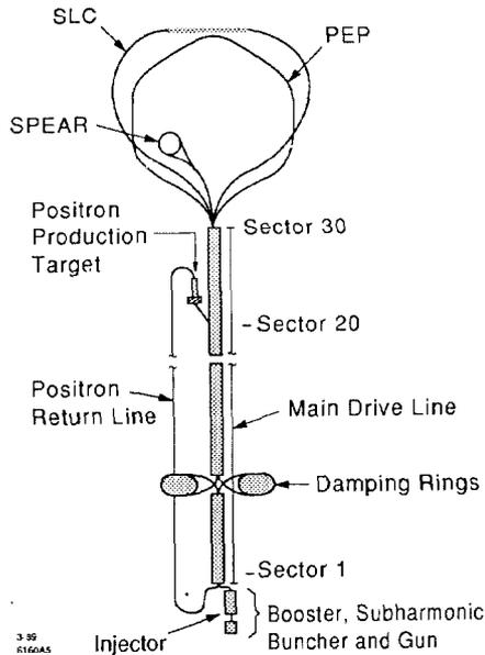
Fig. 1. Schematic layout of the SLAC accelerator complex showing the SLC linac systems including the Damping Rings and off-axis Positron Source, and the PEP and SPEAR storage rings in addition to the SLC ARC's and Final Focus.
