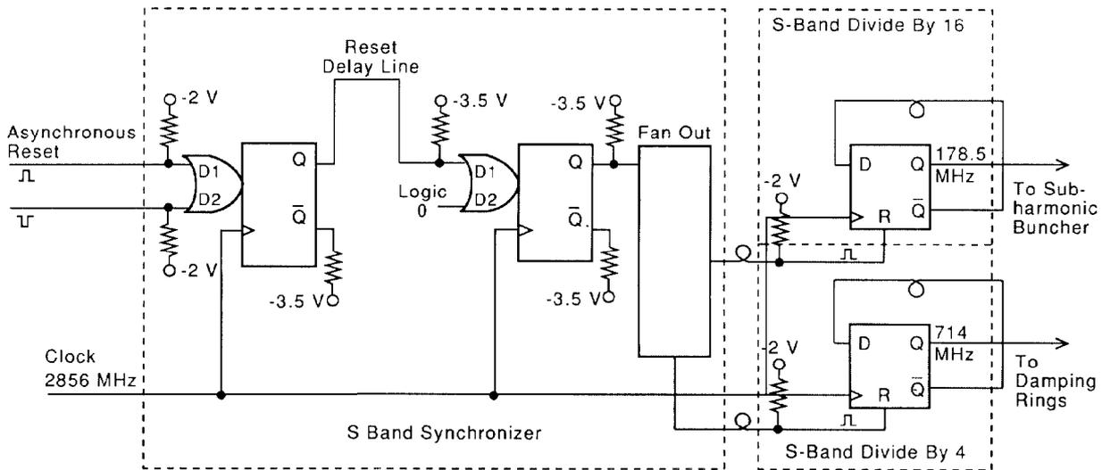
Fig. 4. RF Synchronization electronics block diagram.
