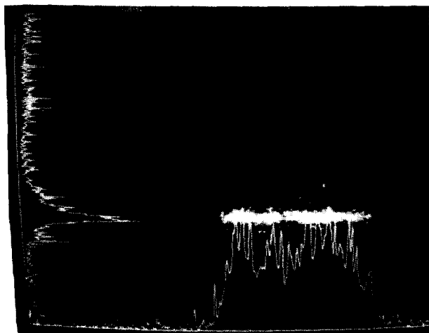
Figure 4: Image of a 25- \mu\text{m} high and 3-mm wide slit collected with an in-beam CCD detector.
