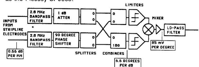
FIGURE 1. Block diagram of the amplitude-to-phase conversion circuit being considered for the new ring closed-orbit system.
