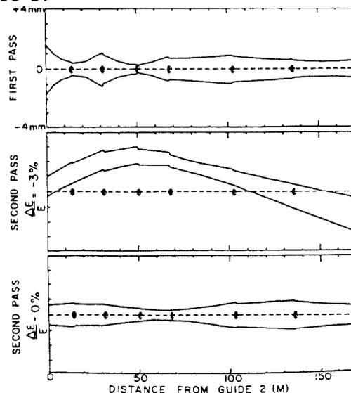
Fig. 2: Computer Simulation of beam envelope using the strong focussing solution for optimizing the energy band pass. The upper trace represents the first pass beam envelope. The lower traces represent the second pass on-energy beam and a beam off-energy by 3%.
