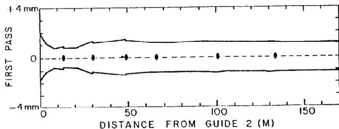
Fig. 1: Computer Simulation of beam envelope using a "weak focussing" solution. Ellipses on axis represent location of quadrupole doublets.
