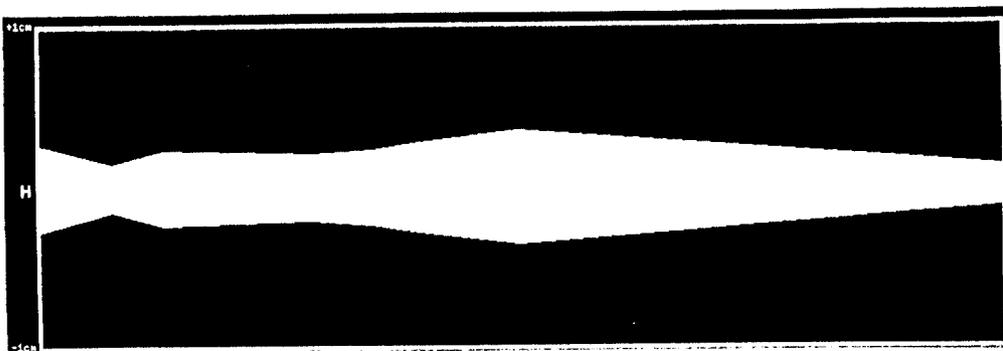
Fig. 6: Measured Horizontal beam envelope in the accelerators.
