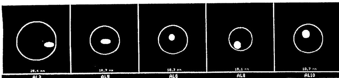
Fig. 7: Horizontal and vertical beam profile information compared with accelerator apertures at different locations in the accelerator.
