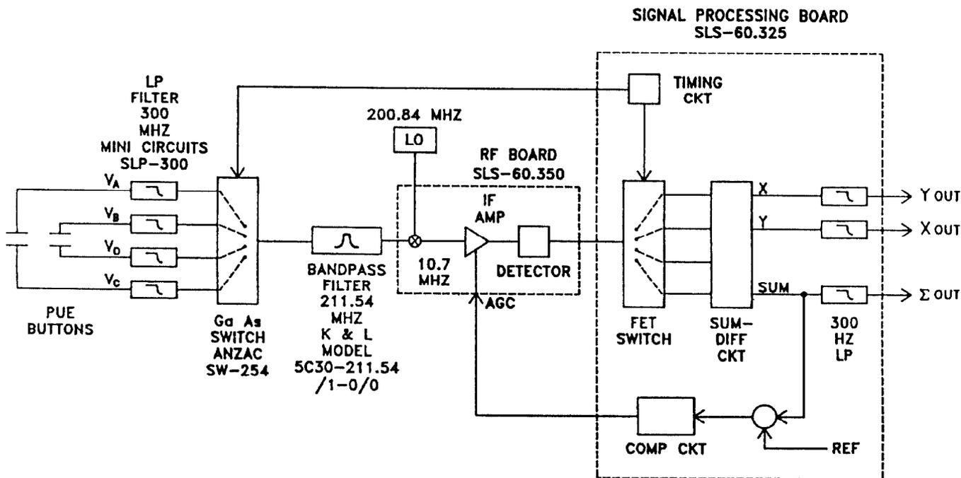
Fig. 2. Block diagram of the switched PUE receiver
