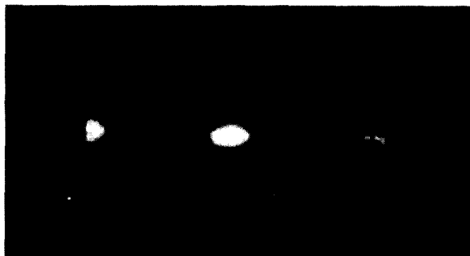
Figure 3: An image of the pinholes at the scintillator screen for the optimum telescope tune. The optimum tune is at a current of 20.5 A. The y axis (vertical) is in the horizontal direction.
