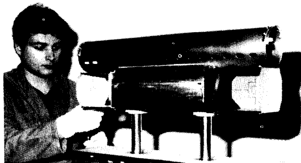
Fig. 5 : Beam stopper block with a circular "RF" chamber. The block is supported on the cooling circuits. On each side of the block is a luminescent screen, which is viewed via a stainless steel mirror.
