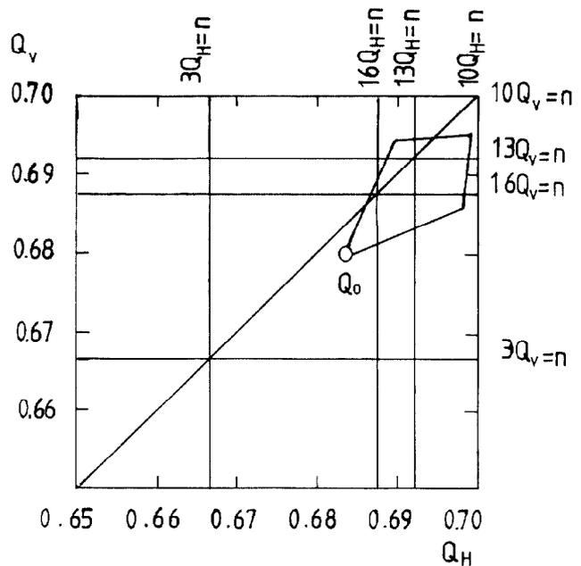
Fig.5: Tune diagram in store. The tunespread for protons and antiprotons in store due to the beam-beam force is similar. At the store energy of 315 GeV the Laslett space charge detuning is negligible.
