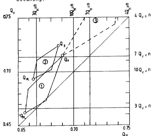
Fig.4) Detuning for different values for the separation in the horizontal plane as a function of the particle amplitude (0 to 5 $\sigma$ ). The separation is given in units of  $\sigma$ .
