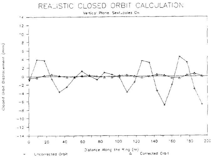
Fig. 2. Vertical incorreted (+) and corrected (Δ) closed orbis for realistic error distribution.
