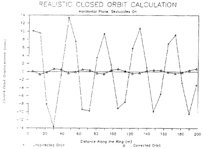
Fig. 1. Horizontal incorreted (+) and corrected (Δ) closed orbis for realistic error distribution.
