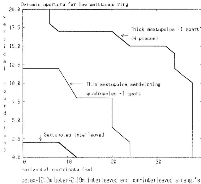
Figure 2: Dynamic aperture of the error-free low emittance ring with various arrangements of sextupoles. See figure 3 for a diagram of the thin-sextupoles-sandwiching-quadrupoles arrangement.
