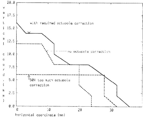
Figure 5: Dynamic aperture with octupoles correcting the effect of the separation of sextupoles sandwiching quadrupoles minus unit matrix apart. betax=12.2m betay=2.13m two pairs of thin sext. 1/2 apart
