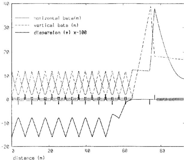
Figure 1: Machine functions for one half of a superperiod. The wiggler is represented as a series of small boxes on the right hand side.
