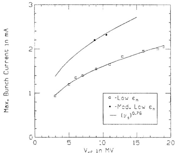
Fig. 1. The maximum single bunch current measured as a function of RF cavity voltage for the low-emittance tune (squares) and the modified low-emittance tune (dots). The curves are the result of a fit to a power law dependence on the synchrotron frequency of  $\nu_s^{0.79}$ .
