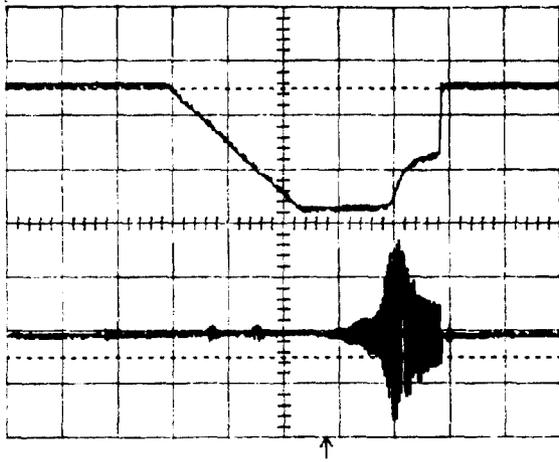
Figure 1. Beam current as a function of time and vertical beam position monitor signals in the PSR. Note the growth of vertical oscillations followed by beam loss.
