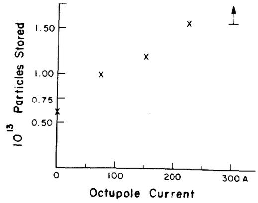
Figure 2. Dependence of maximum stable beam upon various PSR parameters:
