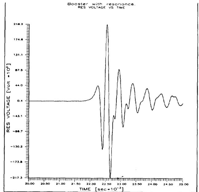
Figure 4: Voltage vs. time induced at one position in the distribution for a "gapped" distribution.
