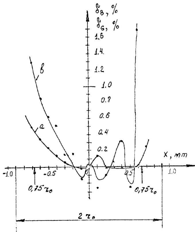
Fig.3. Typical distribution of field nonlinearity (curve a) and gradient nonlinearity (curve b) in the middle of the drift tube. The tolerance for  $r=0.75r_0$  is satisfied.
