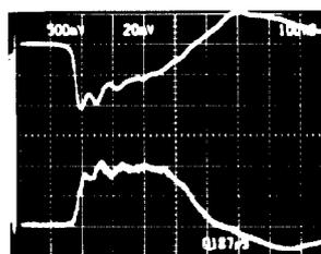
T: diode voltage (162.5 kV/div)
