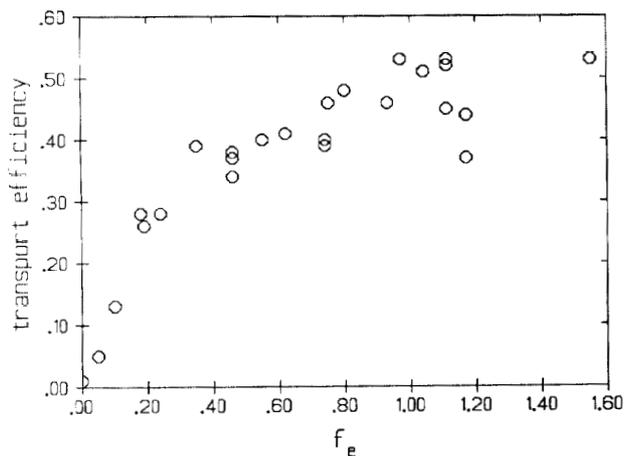
Figure 3. Experimental charge transport efficiency vs.  $f_e$  for Febetron electron beam injection into argon plasma channels.
