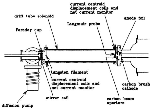
Figure 1. Experimental configuration for electron beam injection into IFR plasma channels.
