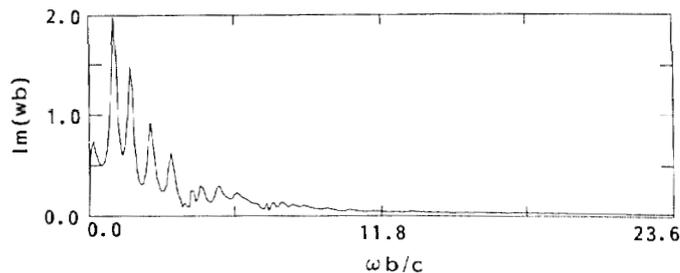
Figure 6. Imaginary part of  $W$  for the shielded line of Fig. 4 with  $b_2/b = 1.33$ ,  $l/b = 2$ ,  $R/b = 3.6$ ,  $d_2/b = 1$ , and  $Z_s = 1$ .
