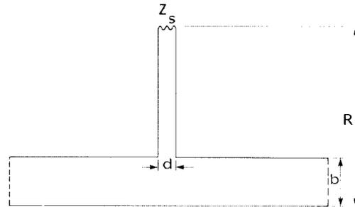
Figure 1. Idealized radial line geometry.
