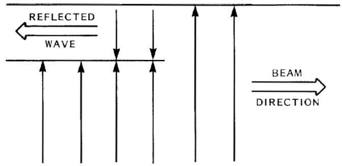
Figure 5. Basic junction between coaxial line and drift tube, showing dipole TE wave launched in coaxial line by field of passing, off center beam.  $E_z$  fields are shown.
