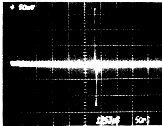
Figure 2. Oscillograph of a single linac micropulse ( \leq 1 ns) produced by a combination of beam chopping at 35 and 750 keV (time: 50 ns/division).
