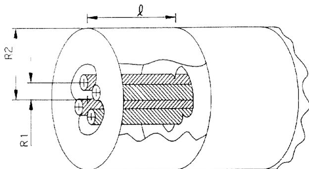
Figure 1: The four-rod cavity RFQ.
