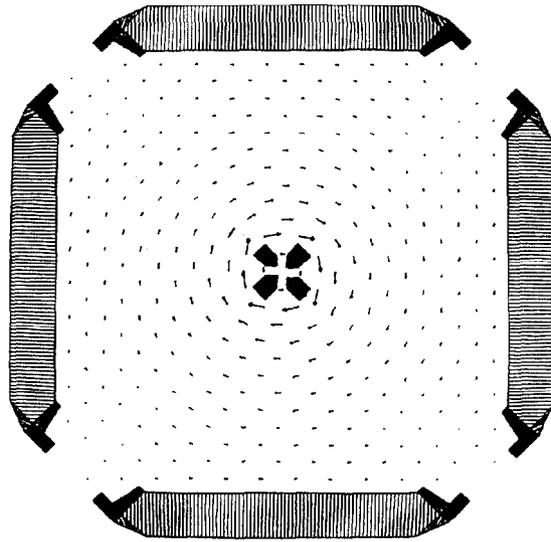
Figure 3: Plot of  $\vec{B}$  for constant  $z$  at the center of a cell.
