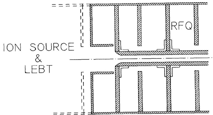
Figure 5: The cross section of the RFQ showing the single gap cavity in front of the RFQ.
