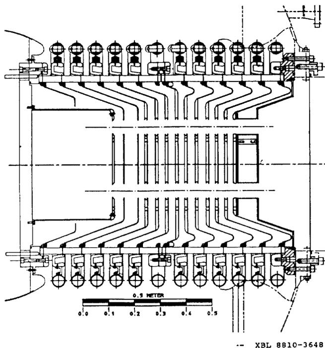
Fig. 4 Acceleration Column Structure.
