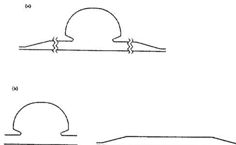
Fig. 2. (a) A complex structure, consisting of an RF cavity and two tapered parts, is decomposed to three components. (b) These components are then recomposed to form two new structures. Both (a) and (b) give the same impedance, while (b) is easy to compute.
