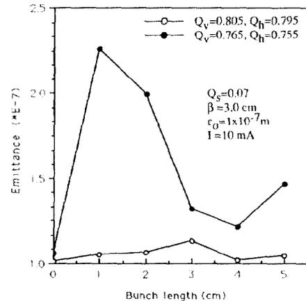
**Fig.4:** Emittance as a function of bunchlength, at two different operating-points.
