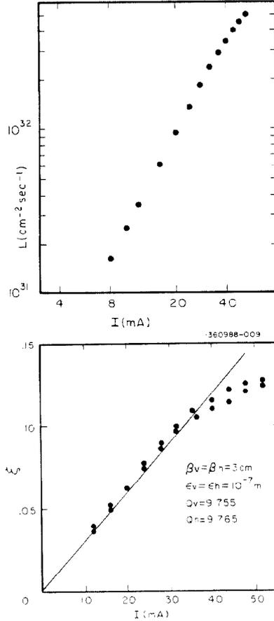
Fig.2: a) Luminosity and b) beam-beam tune shift parameter as a function of single-bunch current for a CESR like round beam machine. Two-dimensional simulation.
