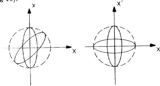
Fig.1: Emittance growth for a)  $\alpha \neq 0$ , and b)  $\beta$  mismatch.
