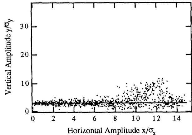
Fig. 4: Identical run to fig. 3 except the longitudinal amplitude of the particles was held to zero. Energy oscillations, chromaticity and horizontal dispersion at the IP are still present.
