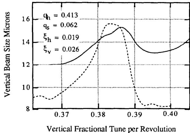
Fig. 1: Weak-beam core size vs. vertical tune. The solid line is experimental data; the dashed is simulation.
