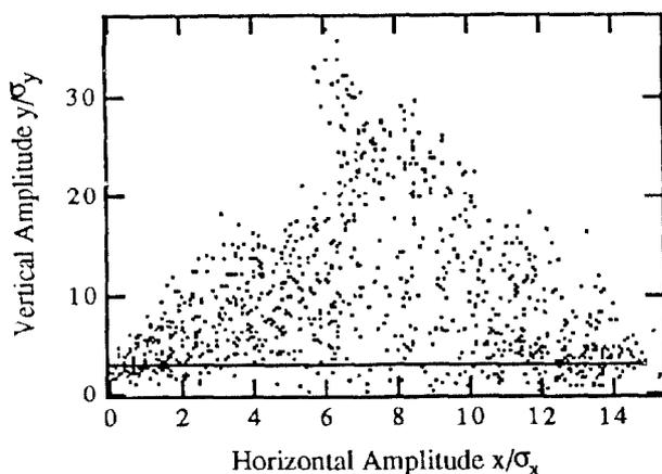
Fig. 3: Ring distribution simulation run with particles initially at amplitudes  $3\sigma_v$ ,  $0.15\sigma_h$ , and  $2\sigma_s$  (3.64cm which is to be compared to  $\beta_v^* = 1.5$ cm). The solid line is the initial distribution; the dots are the final particle positions. The tunes were  $Q_h = 9.410$ ,  $Q_v = 9.380$ , and  $Q_s = 0.062$ . The tune shifts per collision were  $\xi_h = 0.025$  and  $\xi_v = 0.038$ . Only 400 machine turns were tracked.
