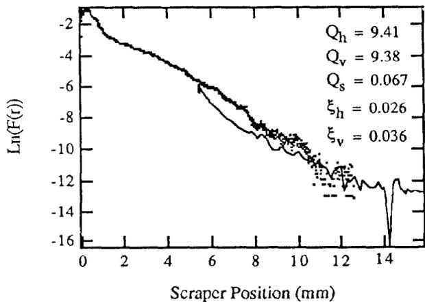
Fig. 2: Logarithm of the distribution  $F(r)$  vs. scraper position from the center of the beam. The dots are simulated data. The solid line is the distribution function reconstructed from the scraper induced lifetime measurements. For this particular case the synchrotron light monitor was accurate out to about the 2mm point, leaving a gap between 2mm and 5.2mm which we were not able to experimentally explore.
