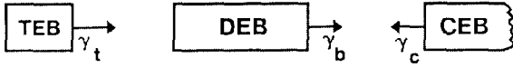
Figure 1. Schematic of the CWFA. The DEB with density n_b \approx n_c/4\gamma_c^2 ( n_c is the CEB density) moves to the right in the CEB (moving to the left) and generate an electrostatic wake that follows the DEB so that a TEB can be loaded on the wake and accelerated to high energy.
