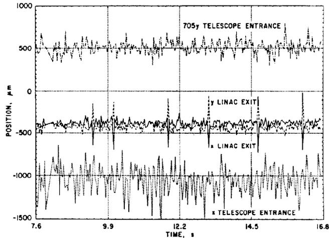
Figure 5: Beam position at linac exit and telescope entrance during the middle 20- $\mu$ s region of the beam, high current.
