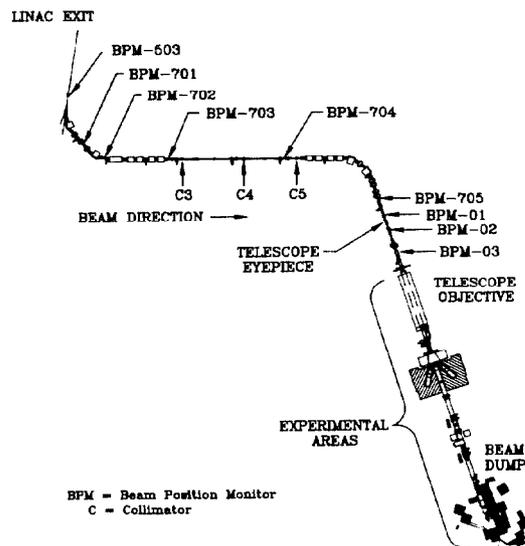
Figure 1: NPBTS line B facility diagram.
