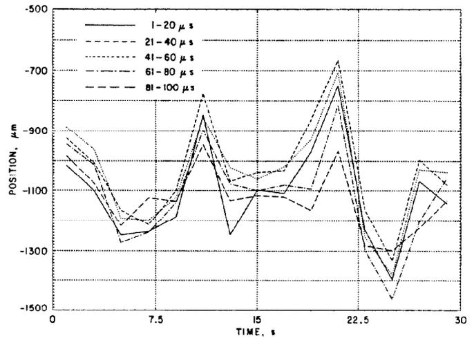
Figure 4: X position at telescope entrance for a portion of the data, high current.
