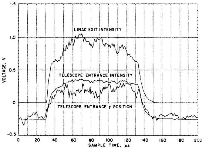
Figure 2: Raw digitized signal from a typical beam pulse from the linac exit intensity output, the telescope entrance intensity output, and the telescope entrance Y position output.
